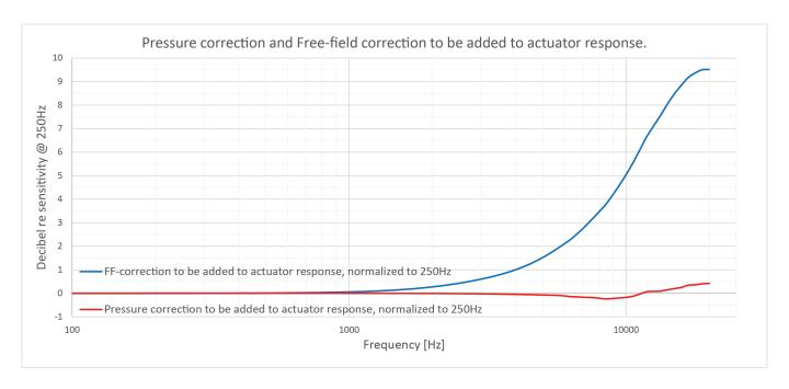
The corrections from actuator to the real pressure and free-field responses
