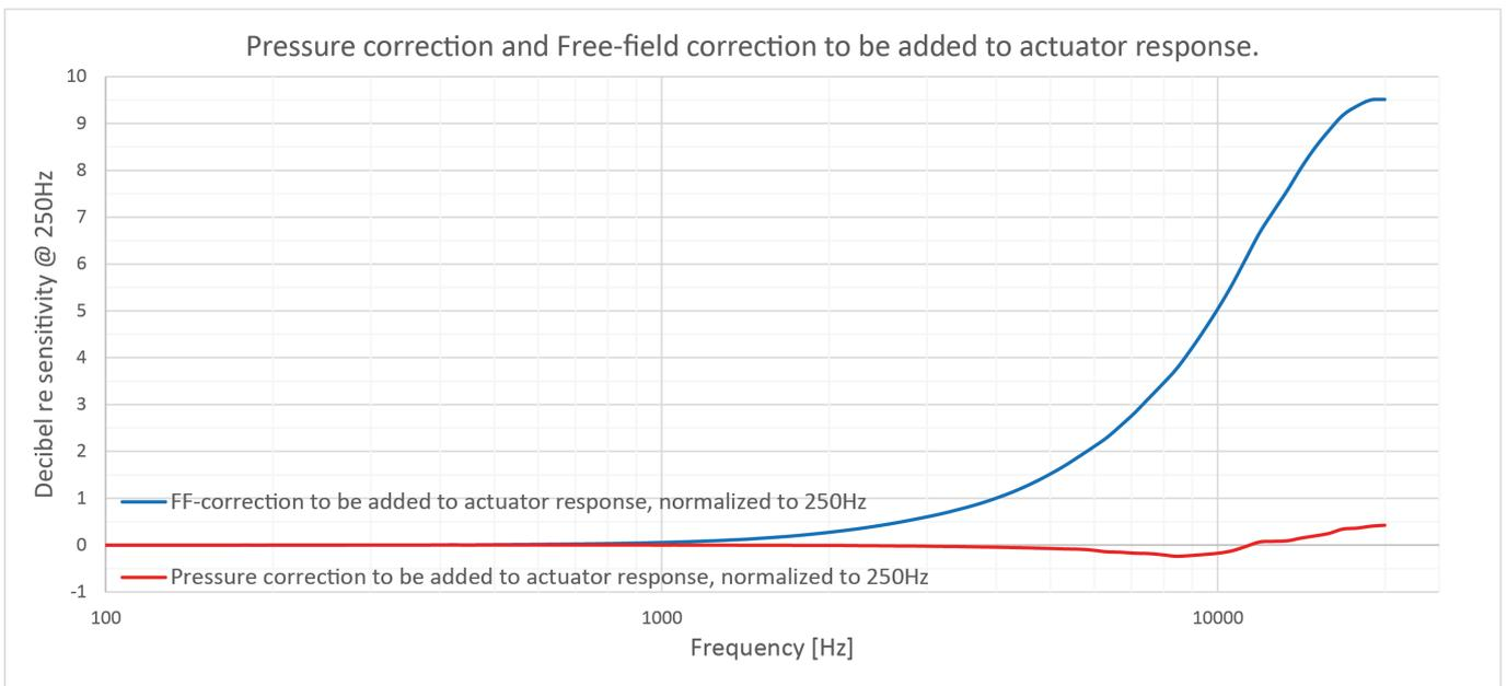
*The corrections from actuator to the real pressure and free-field responses*
