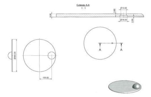
Placement of the microphone in the plate with the windscreen on top. The cutaway of section A to A shows how the microphone fits into the plate.
