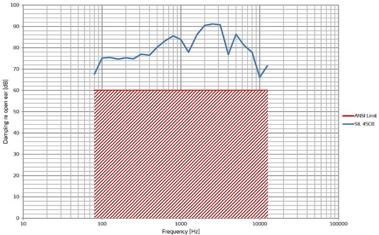
Self Insertion Loss, Measured with closed ear simulators: 100 Hz – 8 kHz >74 dB
