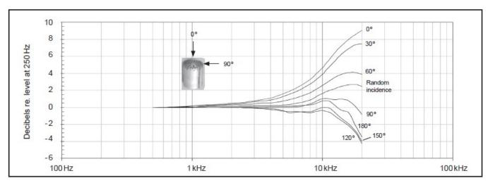
Free-field corrections for different angles of incidence
