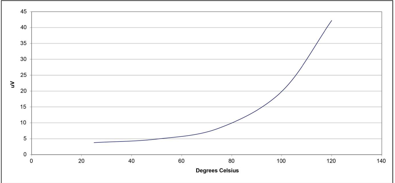
Noise vs. temperature, linear 20 Hz - 20 kHz
