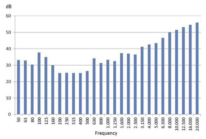
Self Insertion Loss measured in reverberant conditions
