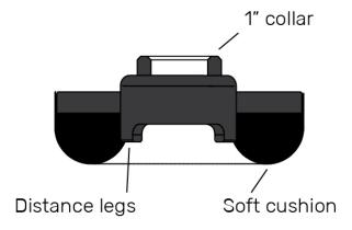
The adapter fits sound calibrators and pistonphones fitted with 1" collar.
