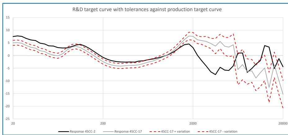
Now we have transferred the target curve from R&D (with ear simulators) to the production environment (ear simulators replaced by microphones) by measuring a typical response with the 45CC-2 microphone configuration. The final step is to introduce upper and lower allowed limits for the frequency response.
