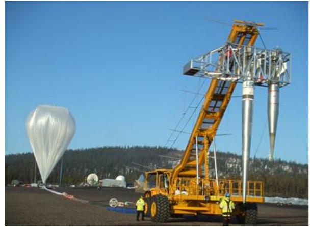
Figure 10: N-WAVE and Low-Boom Models being prepared for drop.
