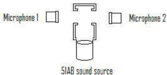
*Figure 1: 51AB calibration - step 1*
