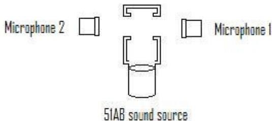
*Figure 2: 51AB calibration - step 2 (Microphones have switched side compared to Fig. 1)*
