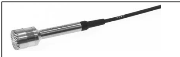
Fig. 5.3 \frac{1}{2} " microphone and \frac{1}{4} " preamplifier to be calibrated
