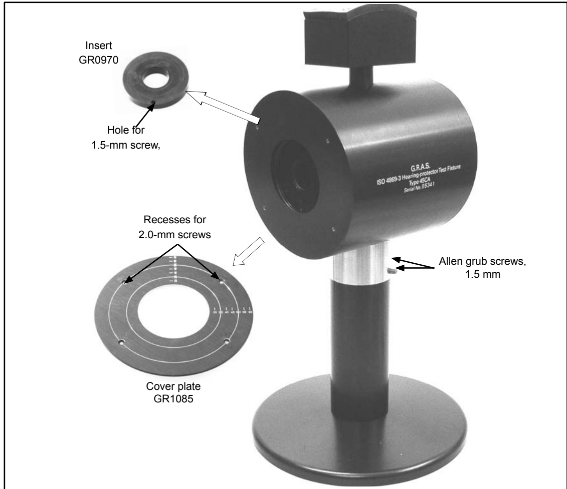
Fig. 6.2 Test-fixture Type 45CA, cover plate and insert removed
