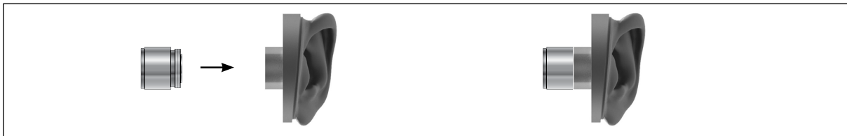
Fig. 6. The pinnae is screw-mounted on the RA0045 Ear Simulator. For clarity, preamplifier and cable are not shown.
