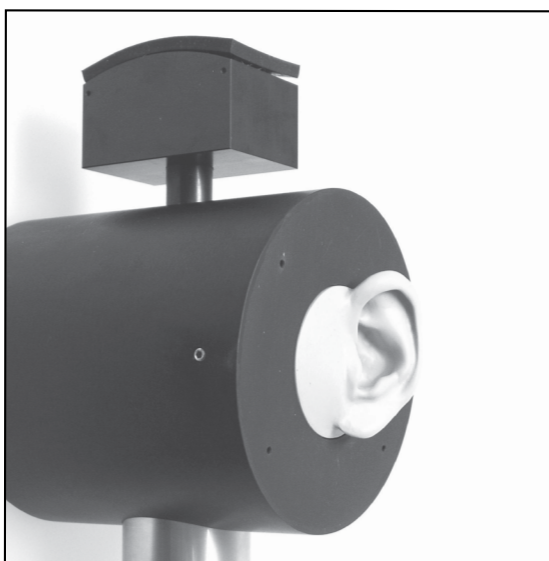
Fig. 4. Mounting the KEMAR pinnae
