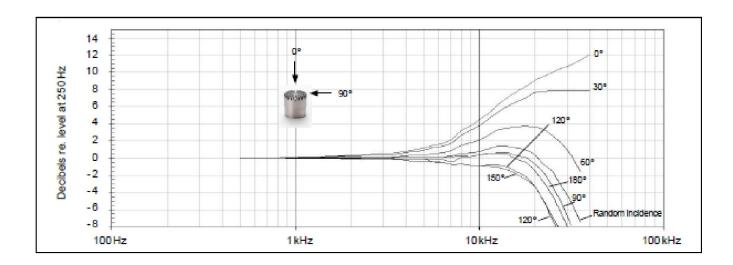
Free-field corrections for various degrees of incidence
