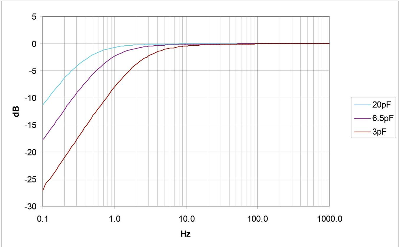
*Typical frequency response for 1/2" (20 pF), 1/4" (6.5 pF) and 1/8" (3 pF) microphones*
