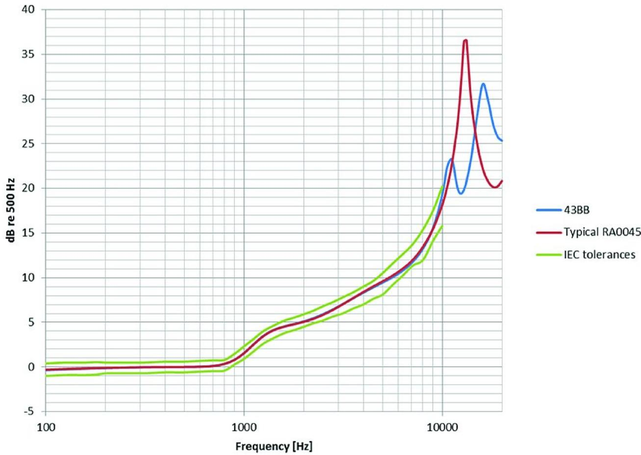
The frequency response is very similar to the standard 60318-4 ear simulator up to 10 kHz
