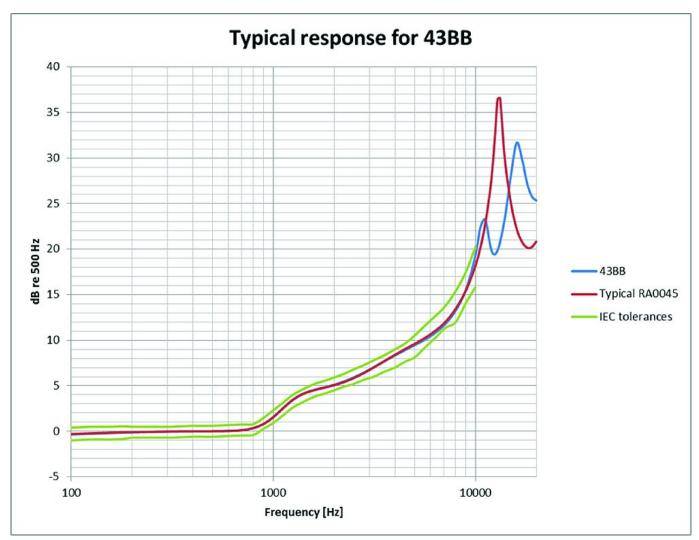
The frequency response is very similar to the standard 60318-4 ear simulator up to 10 kHz
