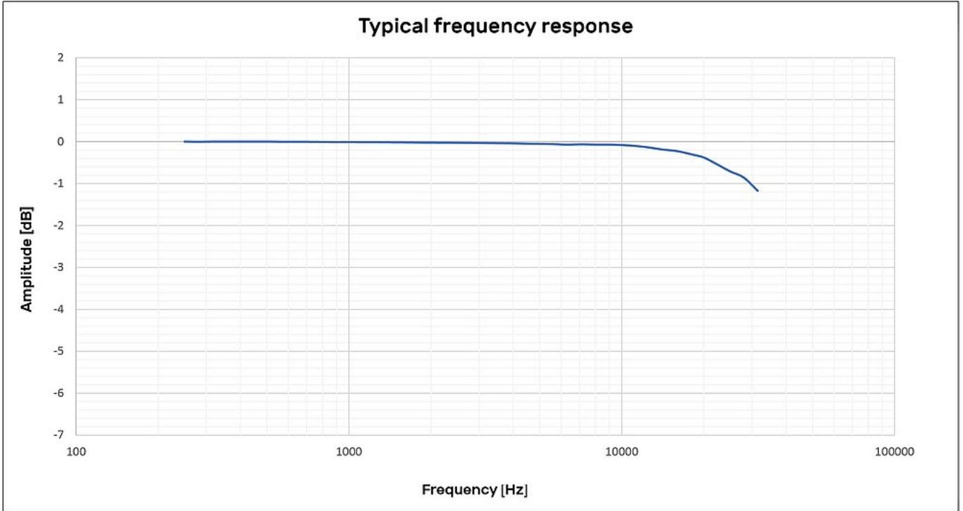
The frequency response is within  $\pm 3$  dB up to 31.5 kHz
